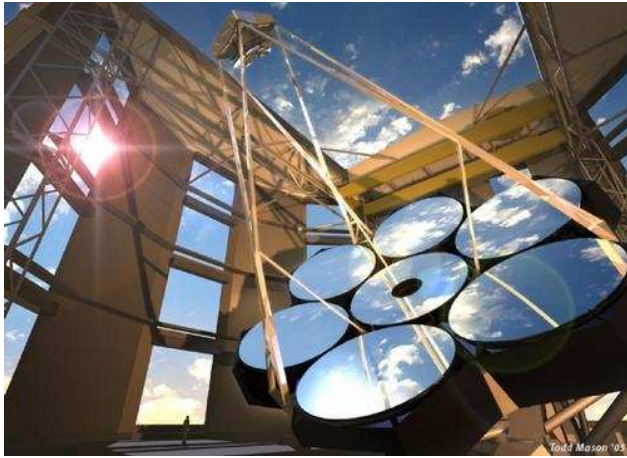
Fig. 5. Artist conception of the design for one of the future giant telescopes that could probe the first generation of galaxies from the ground. The Giant Magellan Telescope (GMT) will contain seven mirrors (each 8.4 meter in diameter) and will have the resolving power equivalent to a 24.5 meter (80 foot) primary mirror. For more details see http://www.gmto.org/
