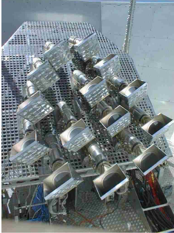
Fig. 8. – The VSA is a dedicated MBR interferometer located at the Observatorio del Teide, Tenerife. Each aperture is about 40 cm in diameter and the table is approximately 3 m across.
